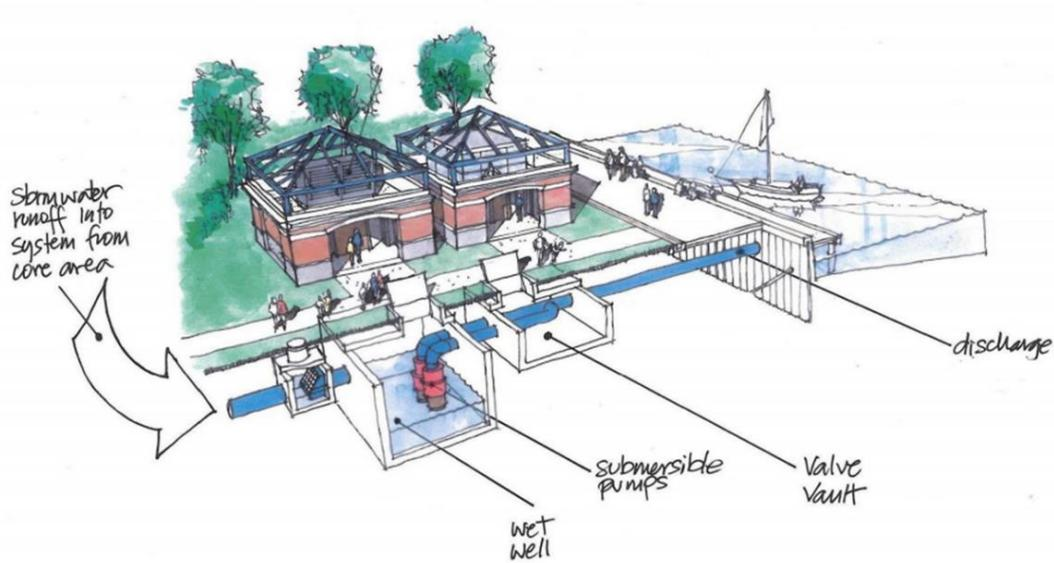
**Figure 4.19** Conceptual Pump Station Schematic (Olin Studios 2012)
